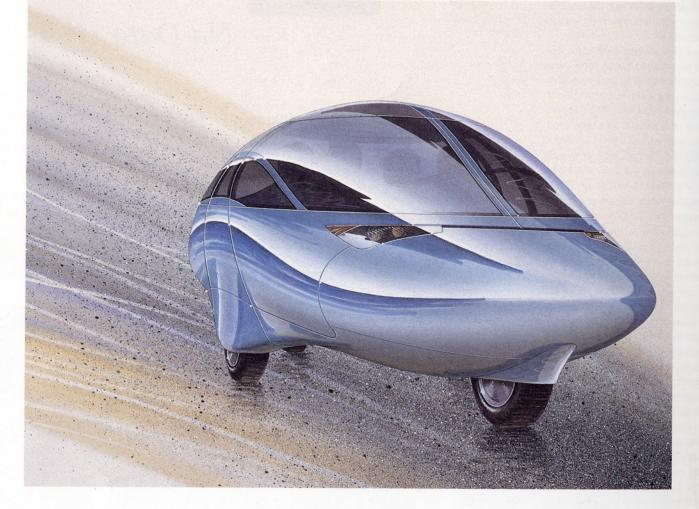
The wheels occupy the four corners of a rhombus. The passengers sit back-to-back, cocooned in what looks like an inverted wing. Petrol consumption is low and wind-tunnel scores are remarkably good (Cw 0,129) The name: lynx. Matthijs van Dijk and Edwin Otten came up with this unusual, albeit not wholly new car concept for their graduate project.
